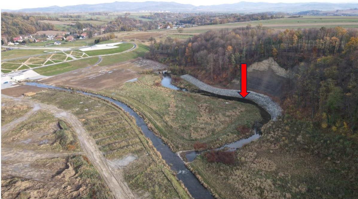
Phot. 16. Visible new section of the inflow channel to the reservoir's dam and preserved section of the Bystrzyca Dusznicka riverbed above the historic bridge (red arrow) (item no. 53 of EMP).
